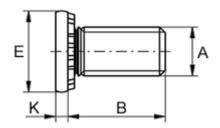
Head diameter E= 8.5Head height K +/-0.02 = 1.50Hole diameter +0.1= 5Length B +/-0.4= 30Male thread A= M5Min distance to edge= 10.5Tightening (N m)= 6.0
